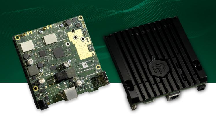
The powerful Wi-Fi 6 radio with MMCX connectors enables further customization: add a HGO-antenna-OUT and you've got yourself an excellent omnidirectional AP... or try the mANT30 PA antenna to create a powerful long-range point-to-point link!
