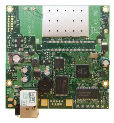
The RB411R is a small CPE type RouterBOARD wireless router with an integrated wireless card.
